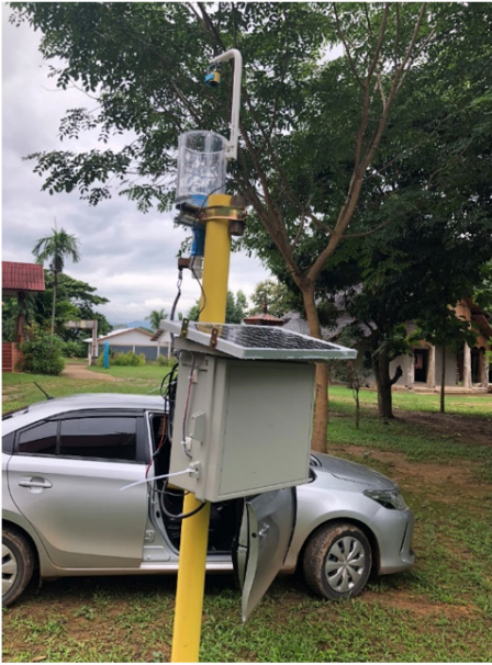
(a) Automatic rain gauges at Wat Phraya Kaeo in Kon watershed
