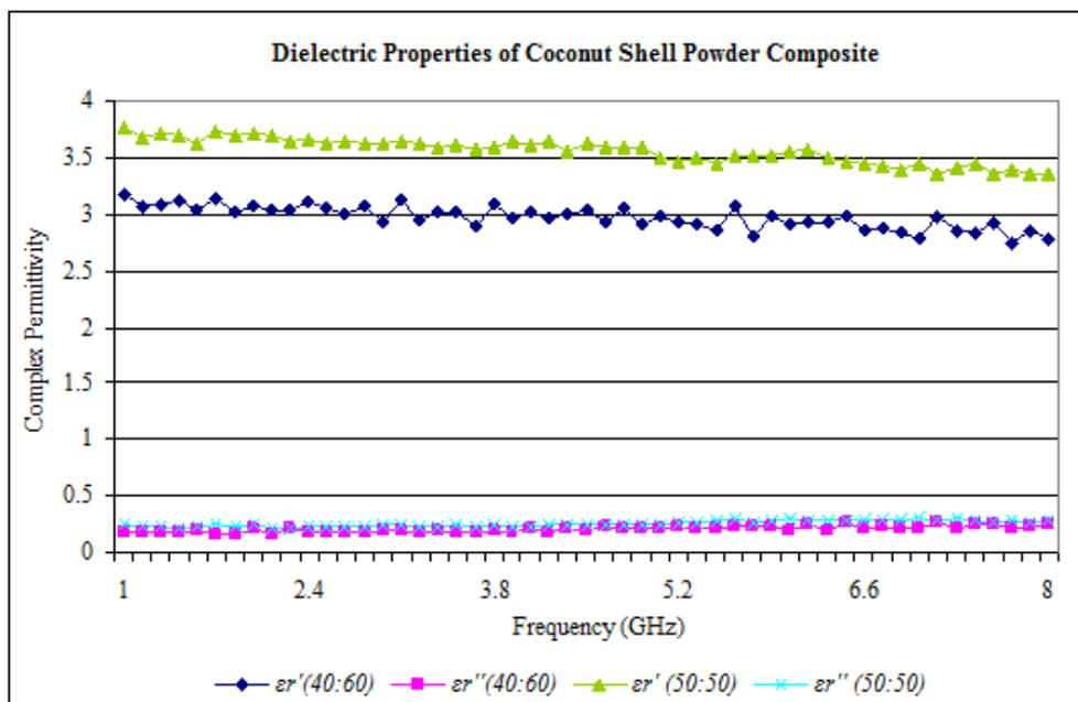
Figure 6. Dielectric properties of coconut shell powder composites
