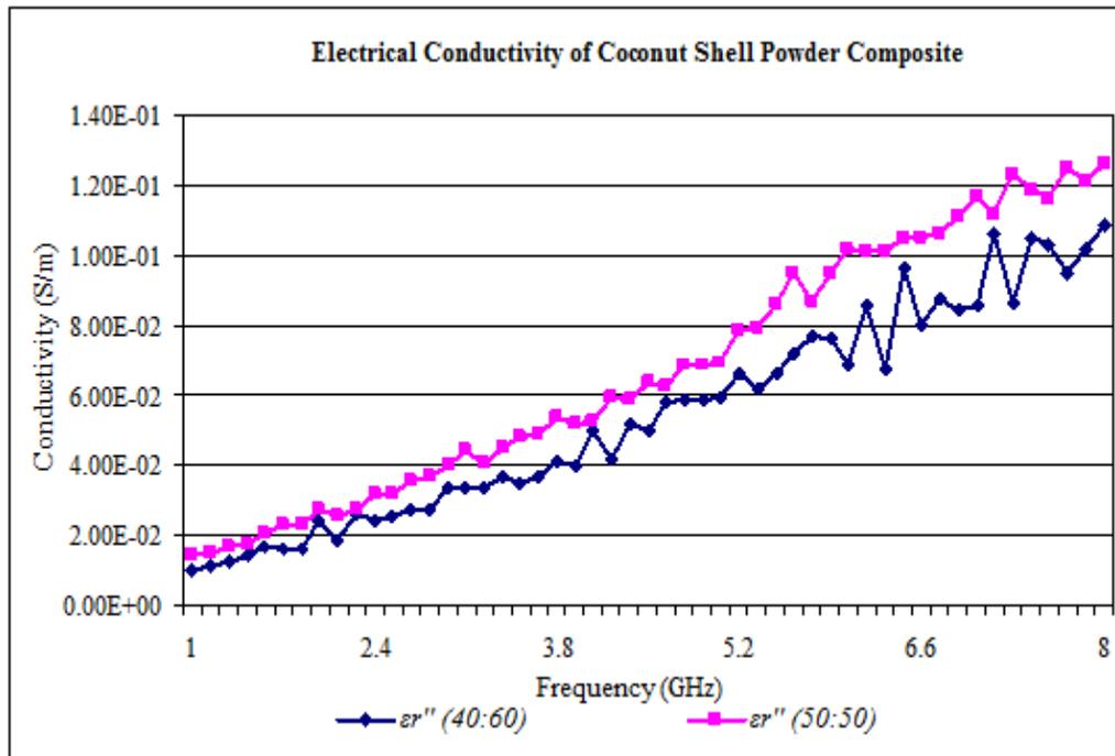
Figure 7. Conductivity of coconut shell powder composites
