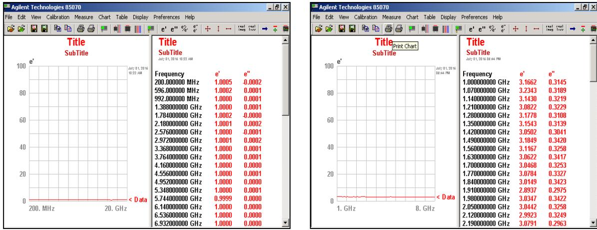
Figure 5. Sample of dielectric properties measurement data (a) Permittivity of air,  $\epsilon_{air} = 1.00$ , (b) Permittivity of CSP composite at frequency 1-8 GHz.
