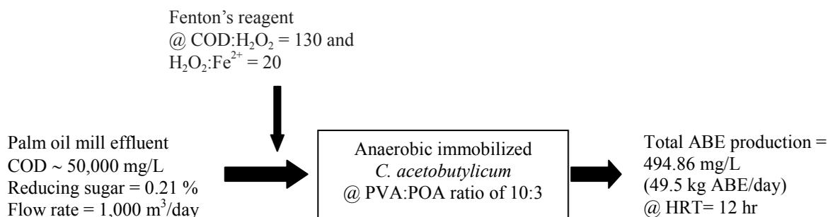
Figure 2. The process summary of ABE production from palm oil mill effluent
