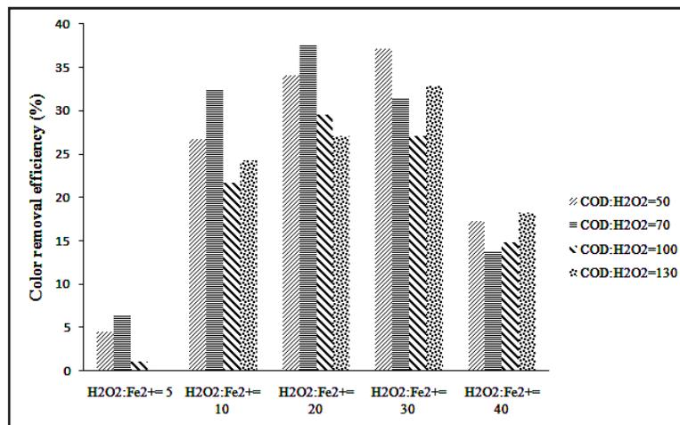
Figure 1. The mean value of color removal efficiency after reacted with Fenton's reagent at different  $H_2O_2:Fe^{2+}$  and COD: $H_2O_2$  ratios
