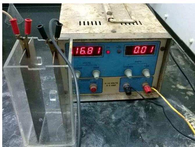
Figure 1. Experimental setup for electrocoagulation
