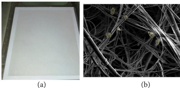
**Figure 6.** a) Colour change-greyness showing soot or black carbon deposition on a glass micro fibre filter paper (Dimensions:  $20.3 \times 25.4 \text{ cm}^2$ ). b) SEM micrograph image depicting size and number of black carbon deposited
